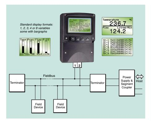
The BA684DF-F Fieldbus Display is a general purpose instrument that can display up to eight fieldbus process variables. Eleven selectable standard screen formats contain one, two, three, four or eight variables, with units of measurement, tag descriptions and bargraphs on some screens.
